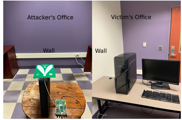
Fig. 6. Setup for the wall-penetrating model extraction attack.
